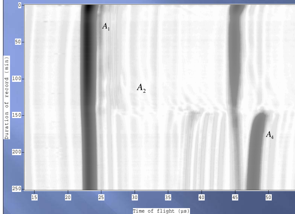
Fig. 12. Superposition of signals Hilbert transforms during hake second defrosting; transducer 5 MHz
