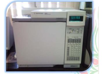
Temperature of the column has ramped from 170 °C to 190 °C in 5 minutes and 0.5 °C per minute and remains in this temperature for 20 minutes
